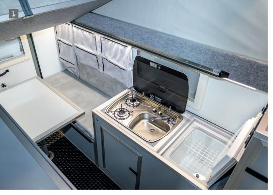
Spacious kitchenette with stainless steel sink, 2-burner gas cooker and cold and hot water connection. Next to it: Top-loader-Engel MB40 cool box (40 l). A freezer (10 l) is located under the fridge.
